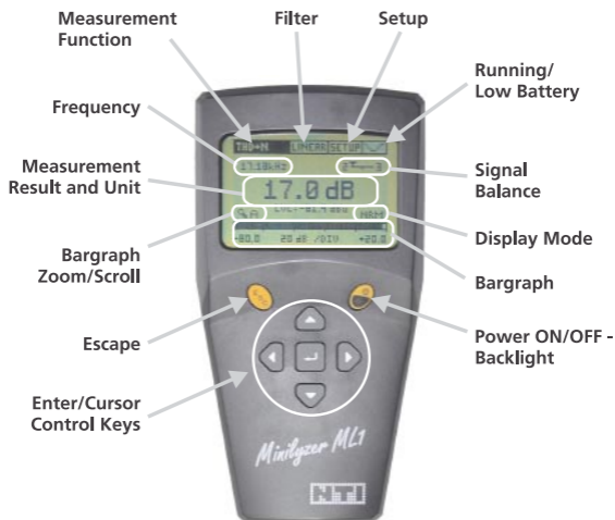
Fig 2.1 Display & Control Elements
