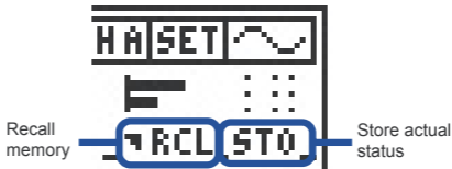
Fig 5-08, Channel status memory field
