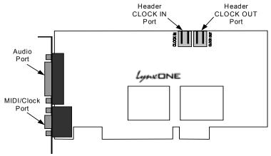
Referring to figure above, locate the Audio Port and the MIDI/Clock Port on the mounting bracket of the LynxONE. Insert the Audio Cable into the Audio Port and tighten the thumb screws on the cable shell. Insert the MIDI/Clock Cable into the MIDI/Clock Port and tighten the thumb screws on the cable shell.
