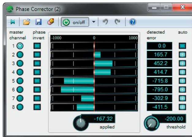
The Phase Corrector allows you to select which tracks are shifted automatically, which are shifted manually, and which (if any) are left unaffected. You can select any channel to be the master channel, and the module will calculate the independent timing errors of all the others, thus allowing you to lock-up the imaging for multitrack, 5.1 and 7.1 material.
