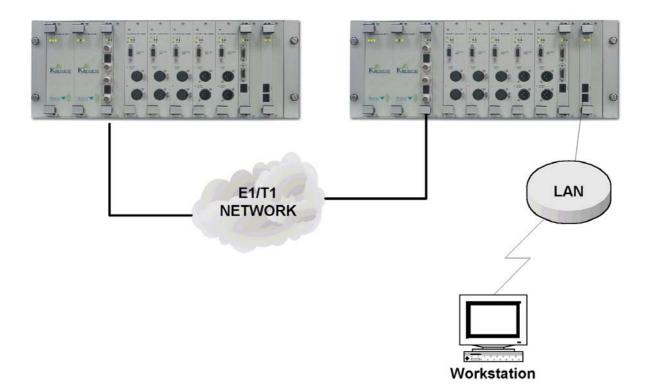
Prodys can supply an application for the management of the Kronos (ProdysControl) it allows access to the control and monitoring functions of the Kronos unit. If you connect a network card (Workstation) to the LAN interface of the Kronos, you must use a cross-over LAN cable.
