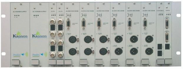
**Kronos** E1/T1 Multiplexer is a system that allows transportation of voice channels, high quality audio and data across 2.048 Mbps or 1544 Mbps structured links (E1 or T1 circuits), using time division multiplexing (TDM). The Kronos multiplexer supports up to four E1 or T1 links. It is possible to drop/insert time slots across any of the connected E1/T1 circuits.
