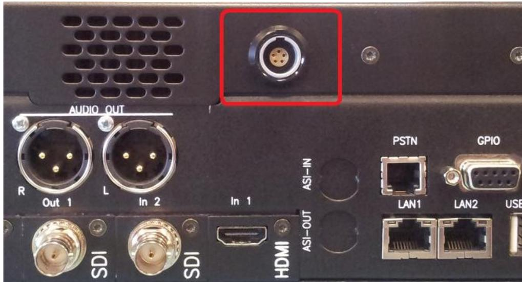
**Picture 17. Rear panel connector for the Wireless Communications Module.**
