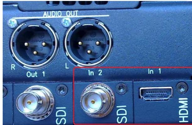
**Picture 14. Video inputs on the rear panel of Ikusnet Portable**
