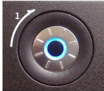
Press softly on the round control and turn it to the left or to the right to decrease or increase the gain. To balance the relative level of the Tx and Rx audio signals **press again the middle button, the L and R' leds will start blinking, indicating that the current audio level configuration is to balance the relative levels of Tx and Rx signals.** The display will show the relative level as in the examples below:
