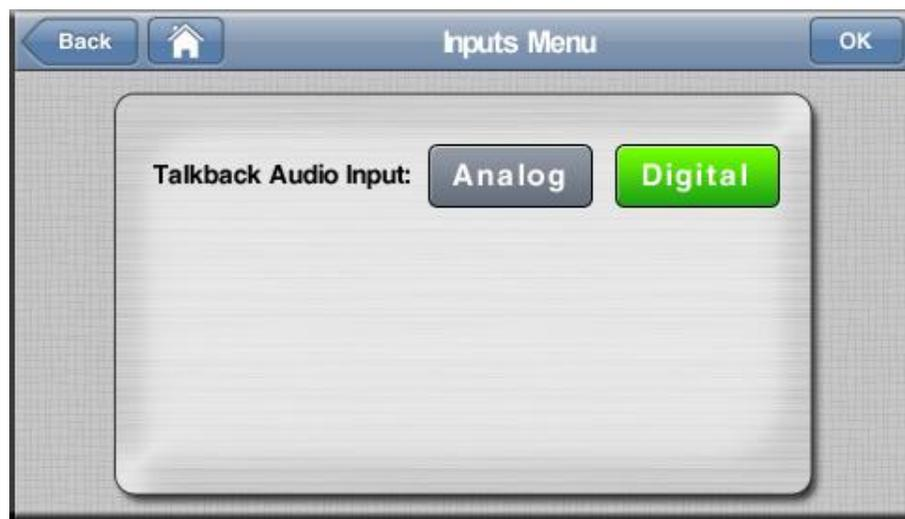
**Picture 75. Audio inputs menu for Ikusnet ST.**
