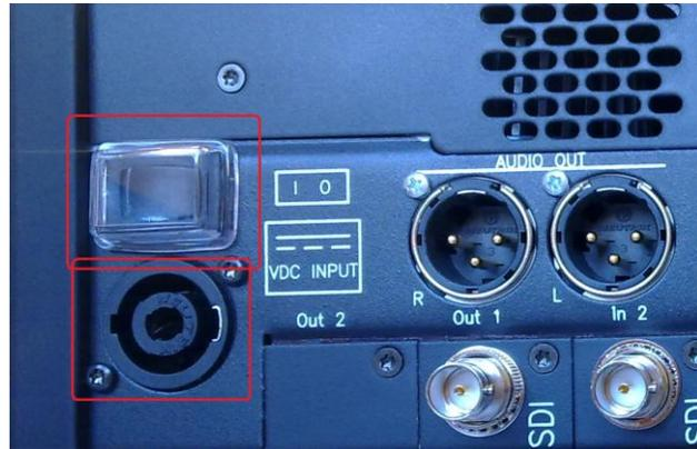
**Picture 9. Ikusnet Portable Power switch and power inlet**
