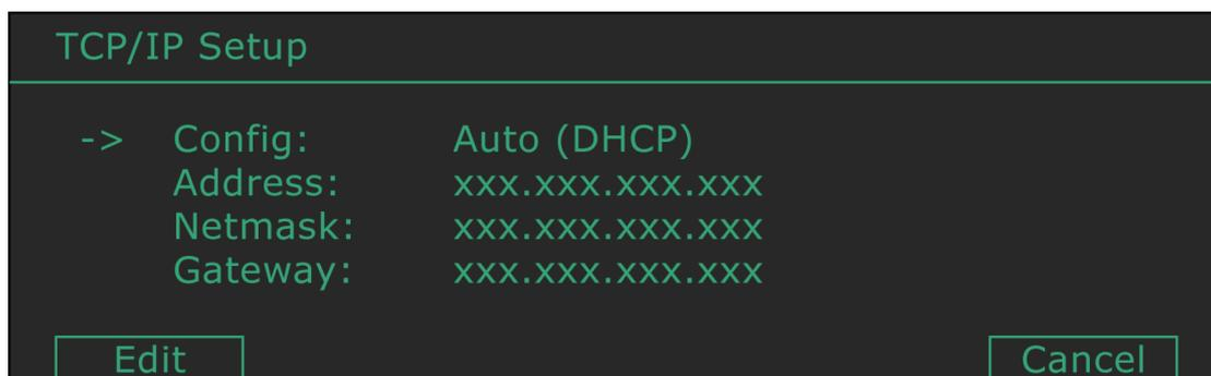
The network interface may be configured automatically if your network has a DHCP server, or manually. Toggle between these states by pressing EDIT when the Config menu item is indicated.
